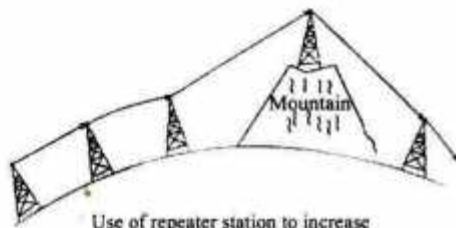
Use of repeater station to increase the range of communication
