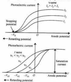
If radiations of same frequency v but different intensities  $I_1$  and  $I_2$  are incident on metallic surface, then it is found that photoelectric current produced is different but stopping potential  $V_0$  is same. As maximum kinetic energy with which photoelectrons are emitted is proportional to stopping potential  $V_0$ , so it follows that maximum kinetic energy with which photoelectrons are emitted is independent of intensity of incident light.
