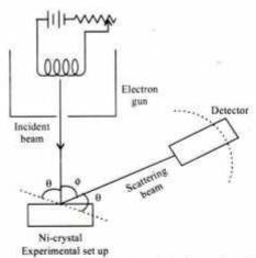
For different values of scattering angles, intensity of scattered beam of electrons is measured.
