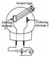
A photo-cell converts a change in intensity of light into a change in photoelectric current. This current can be used to operate control systems and in light measuring devices.
