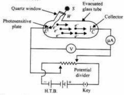
"The retarding potential  $V_0$  at which no photo electron reaches the collecting electrode C and the photoelectric current in the circuit becomes zero is called "stopping potential".
