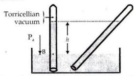
A long glass tube (of about 1 m length) closed at one end was filled completely with mercury and then was inverted in a trough containing mercury.
