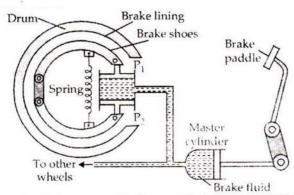
a small force applied over the brake paddle is transmitted by the brake fluid as a large force to the piston for brake and as a result, the brake shoes open tend to up. They press against the brake linings of the drums of the wheels and bring them to rest.
