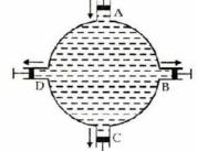
The pistons B, C, D move outwards travelling the same distances. To stop the motion of these pistons, we have to exert equal force on each piston; the magnitude of each force being equal to the force applied on piston A. It means that the pressure is transmitted by the liquid equally, undiminished in all directions.
