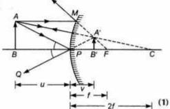
Let convex mirror form virtual, erect diminished image A'B' on the other side of mirror of an object AB as shown in above figure.
