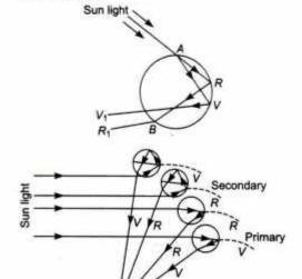
The primary rainbow is formed by those rays which suffer one total internal reflection and two refraction and comes out of the rain drop at angle of minimum deviation.
