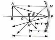
(1) Let an object AB is placed at a distance u from the concave mirror and its real inverted image form at a distance from it. C is centre of curvature of mirror.
