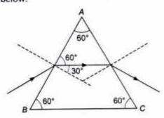
By geometry Angle of refraction  $r = 30^{\circ} (1/2)$
