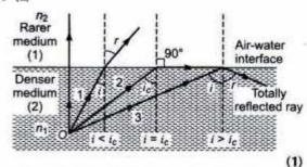
The critical angle is that angle of incidence in denser medium for which the angle of refraction in the rarer medium is 90° as shown by ray 2.
